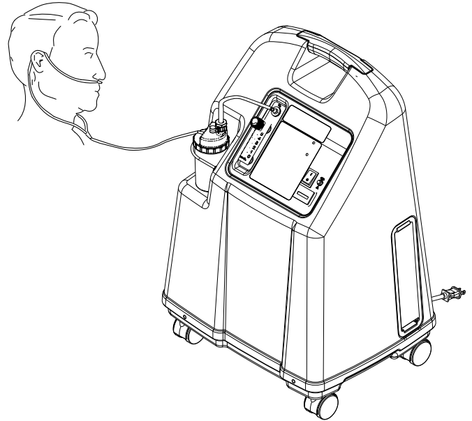
Fig. 4-2 Concentrator with Humidifier
