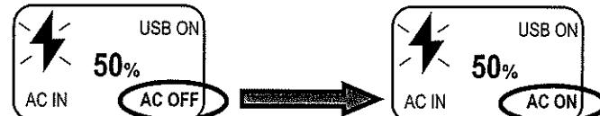
When using as an Uninterruptible Power Supply (UPS), set-up your CPAP or BiPAP device as shown below. While receiving therapy, the battery stays charged.
