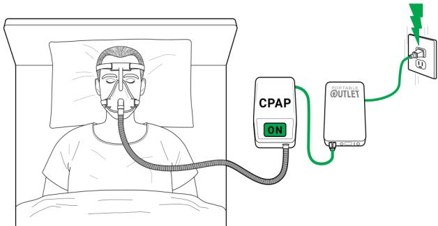
**When there is an outage, the battery switches ON.**
