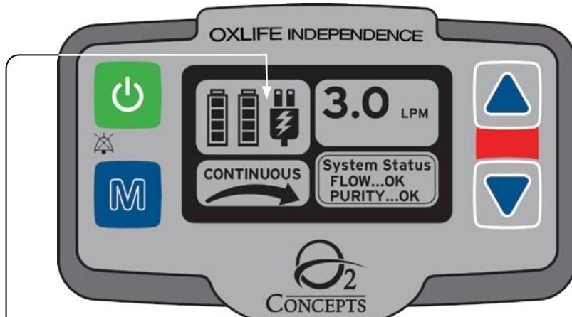
THE EXTERNAL POWER SOURCE ICON WILL BE DISPLAYED ON THE CONTROL PANEL.
