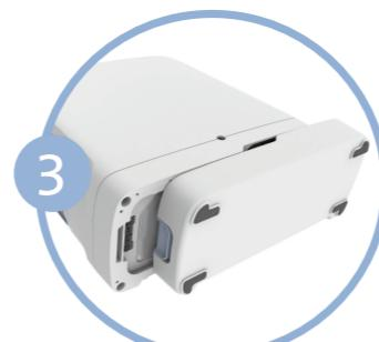
Remove the battery from the Inogen One® G5/Rove 6 concentrator.
