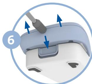
6 Press battery latch down and slide charger off battery.
